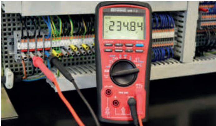
mains voltage measurement with AutoV and LoZ function
