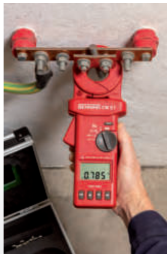
Measuring the earth loop resistance of an installation's earth connection
