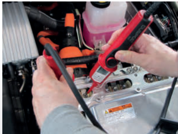
Testing the high DC voltage of a HV electric vehicle
